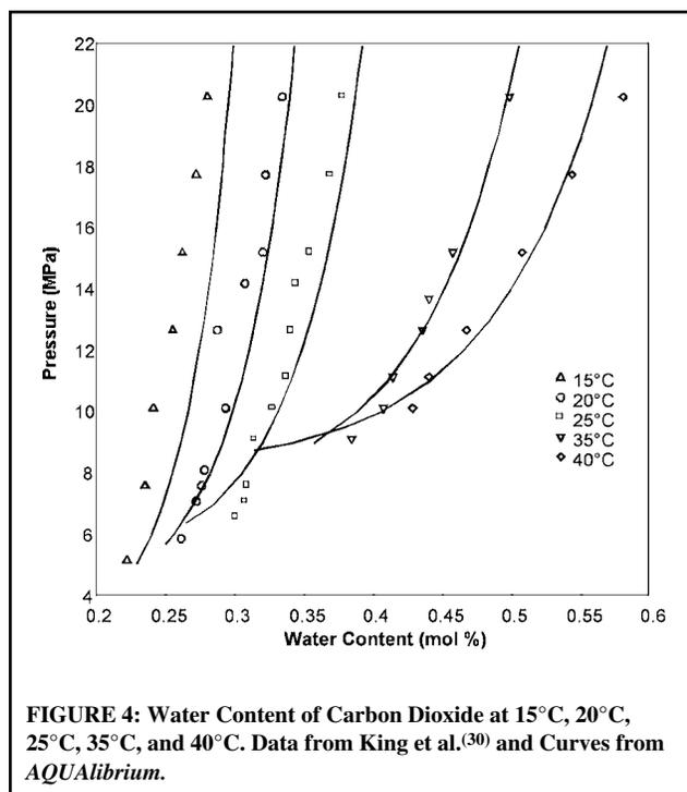
FIGURE 4: Water Content of Carbon Dioxide at 15° C, 20° C, 25° C, 35° C, and 40° C. Data from King et al.<sup>(30)</sup> and Curves from AQUALibrium.
