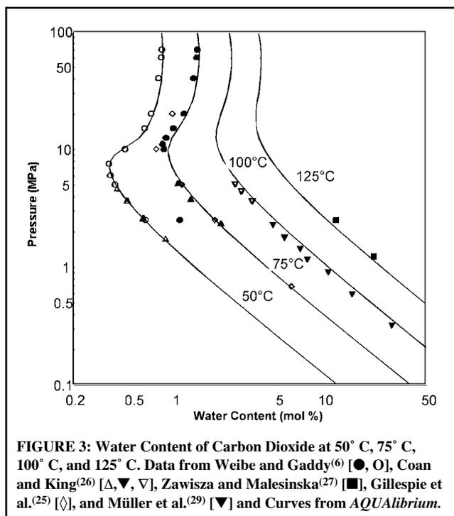
FIGURE 3: Water Content of Carbon Dioxide at 50° C, 75° C, 100° C, and 125° C. Data from Weibe and Gaddy<sup>(6)</sup> [●, ○], Coan and King<sup>(26)</sup> [Δ, ▽, ▽], Zawisza and Malesinska<sup>(27)</sup> [■], Gillespie et al.<sup>(25)</sup> [◇], and Müller et al.<sup>(29)</sup> [▼] and Curves from AQUALibrium.
