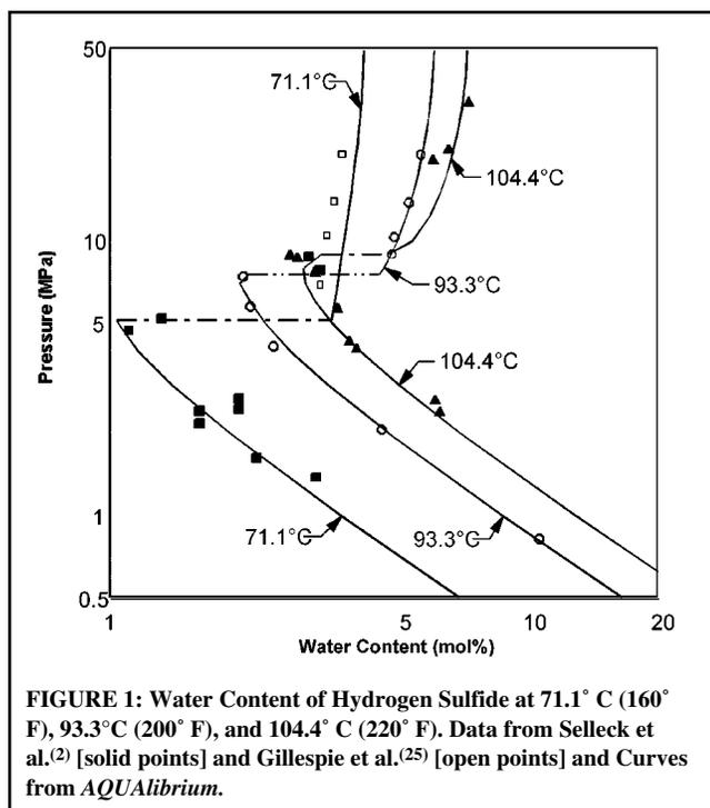
**FIGURE 1: Water Content of Hydrogen Sulfide at 71.1° C (160° F), 93.3° C (200° F), and 104.4° C (220° F). Data from Selleck et al.<sup>(2)</sup> [solid points] and Gillespie et al.<sup>(25)</sup> [open points] and Curves from *AQUALIBRIUM*.**
