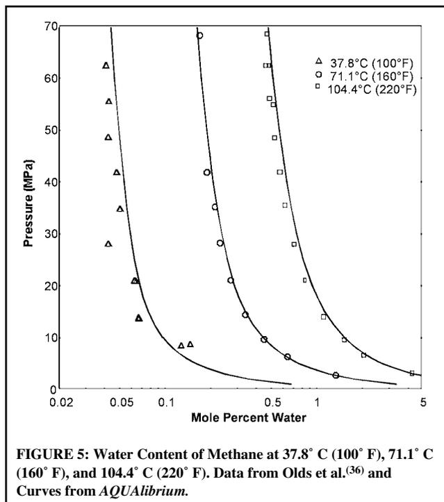
FIGURE 5: Water Content of Methane at 37.8° C (100° F), 71.1° C (160° F), and 104.4° C (220° F). Data from Olds et al.<sup>(36)</sup> and Curves from AQUALibrium.
