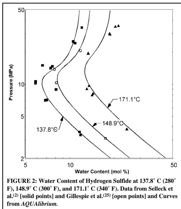
**FIGURE 2: Water Content of Hydrogen Sulfide at 137.8° C (280° F), 148.9° C (300° F), and 171.1° C (340° F). Data from Selleck et al.<sup>(2)</sup> [solid points] and Gillespie et al.<sup>(25)</sup> [open points] and Curves from *AQUALIBRIUM*.**
