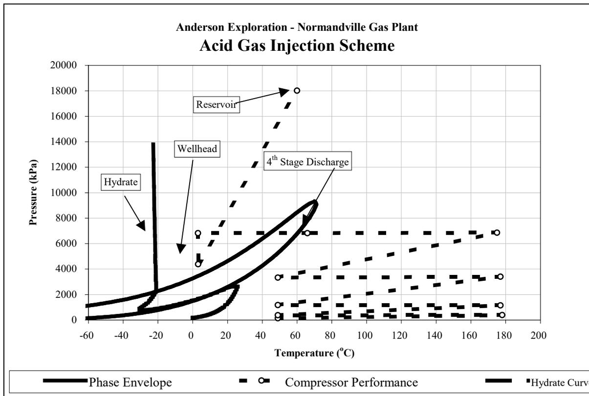
The final predicted hydrate temperature is approximately -22°F (-30°C), substantially colder than the line would get during normal injection operations.
