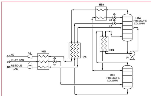
Figure 3. Double column process (DBLC process).
