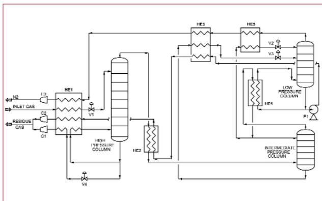
Figure 4. Three column process (3COL process).
