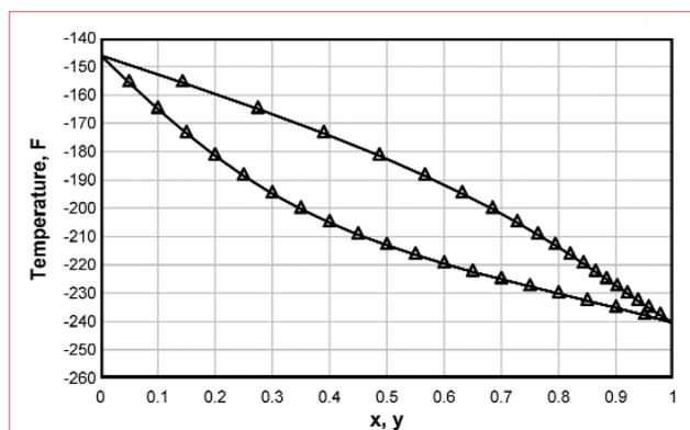
Figure 1. T-x-y curve for N<sub>2</sub>-CH<sub>4</sub> at P=400 psia.
