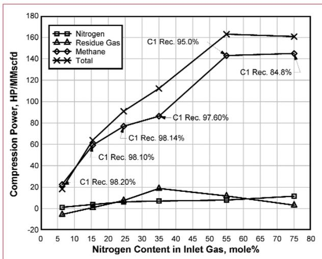
Figure 6. Total and component compression power for single column process.
