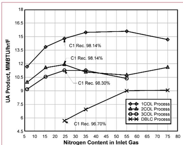
**Figure 11. UA product for four nitrogen removal processes.**
