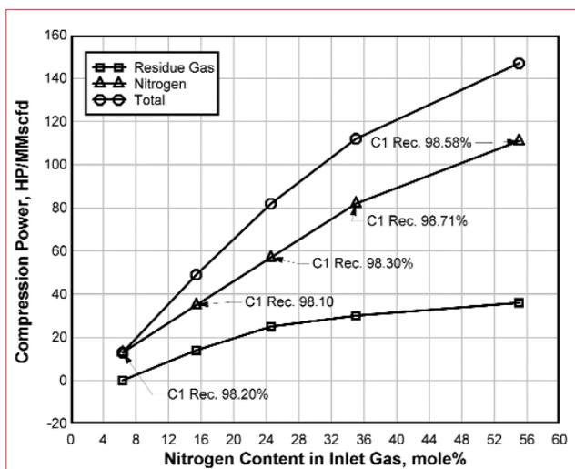
Figure 8. Total and component compression power for three column process.
