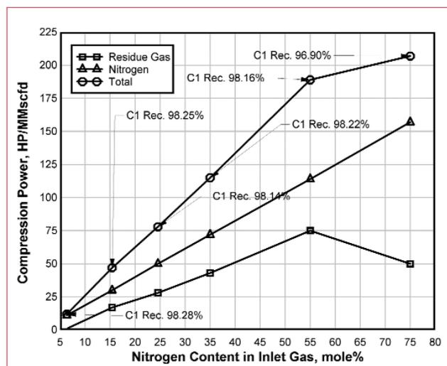
Figure 9. Total and component compression power for two column process.
