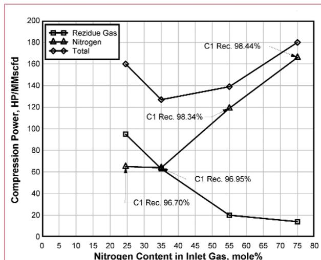
Figure 7. Total and component compression power for double column process.
