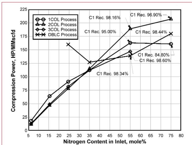
**Figure 10. Total compression power for four NR processes.**
