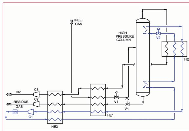
Figure 2. Single column process (1COL process).
