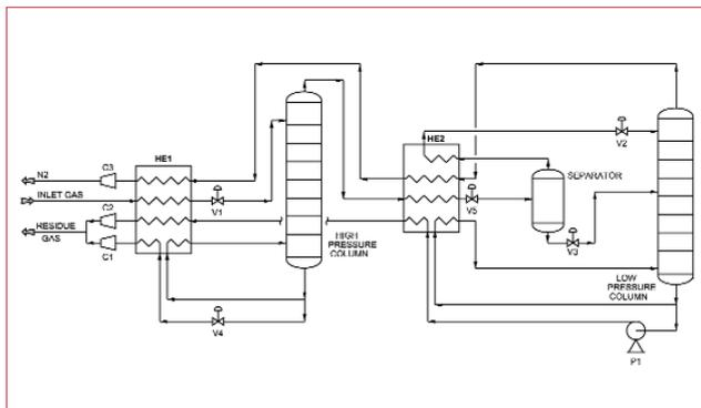
Figure 5. Two column process (2COL process).
